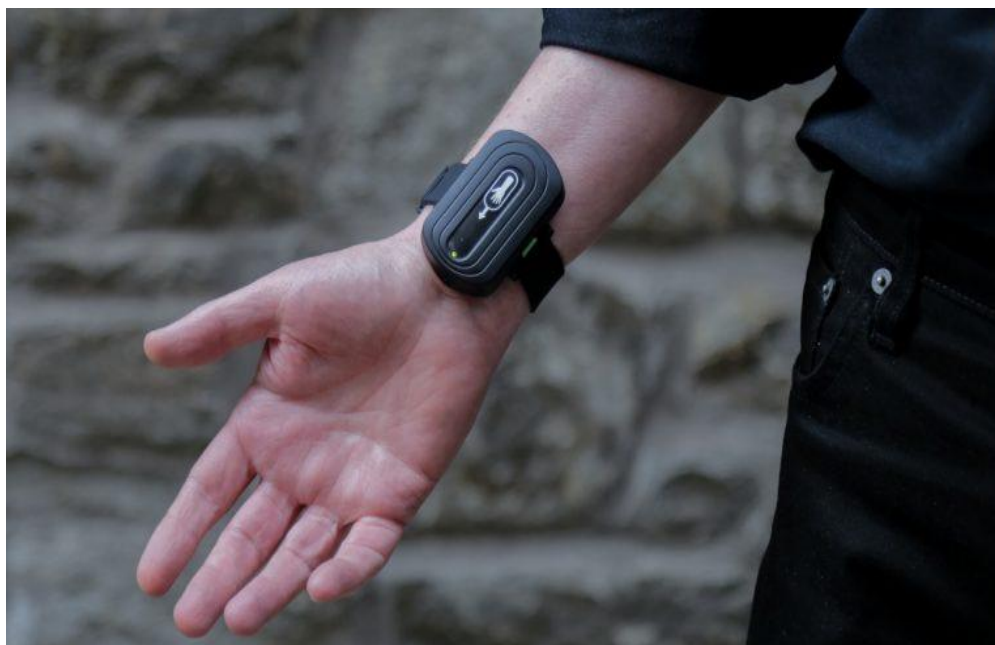
Figure 2. Neupulse is a wearable device that stimulates the median nerve in the wrist. Image credit: Kinneir Dufort. [41]. The median nerve is a major nerve that provides both motor and sensory functions to the forearm, wrist, and hand. The relationship between the median nerve and TS is still being studied, and more research is needed to fully understand any potential connections. The goal is for Neupulse to be available to the Tourette's community globally in the years ahead.
