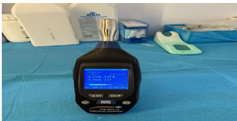
Figure 1. PCE-MPC 10 particle counter used for measuring PM 2.5 and PM 10 concentrations in clinical settings, specifically within the assistant area.
